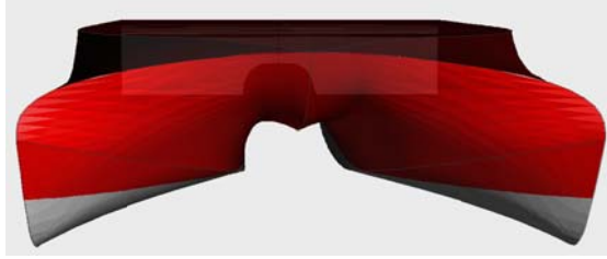
Gambar 13. Konfigurasi Model 9 ( B_{Hull} = 3,50m outer flat hull)
