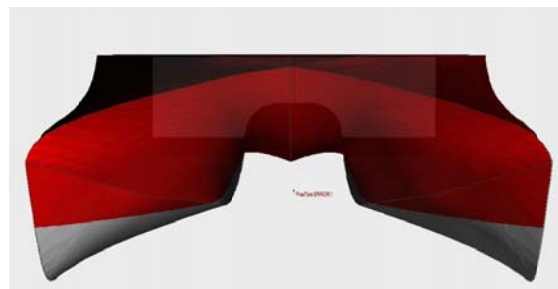
Gambar 12. Konfigurasi Model 8 ( B_{Hull} = 3,00m outer flat hull )
