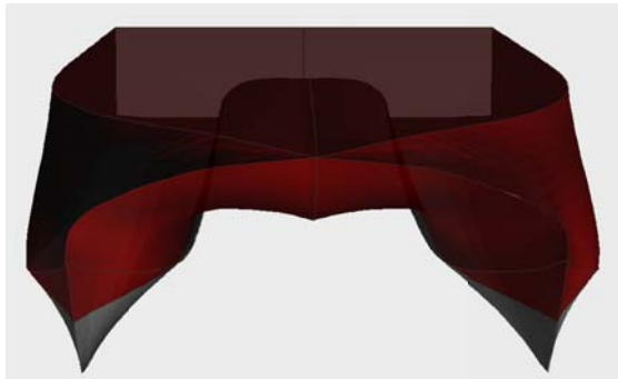
Gambar 8. Konfigurasi Model 4( B_{Hull} = 2,50m symetri hull )
