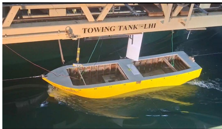
Figure 10. Ship model with wing sail installed during the wind-assisted resistance test
