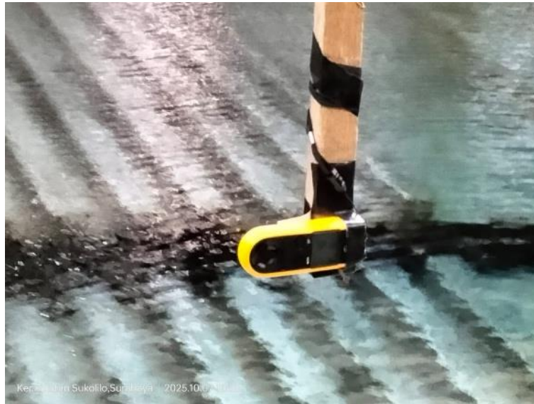
Figure 9. Portable anemometer mounted at the base of the wing sail mast
