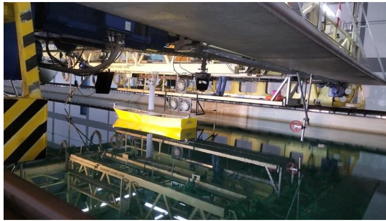
Figure 6. Resistance test at Towing tank
