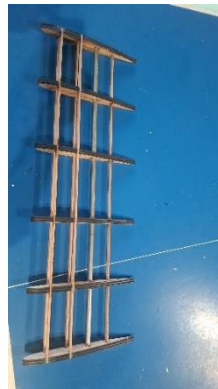
Figure 4. Wing sail model with NACA 0015 airfoil profile
