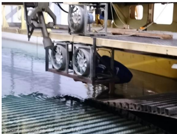
Figure 8. Blower unit mounted on the towing carriage
