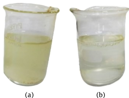
Figure 7. Photo of liquid tofu waste (a) before filtration (b) after filtration
