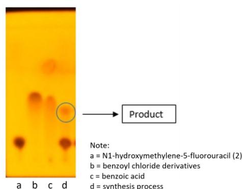
**Figure 2.** TLC spot of synthesized 5-Fu derivatives
