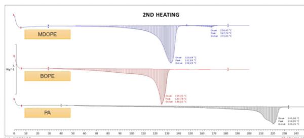
**Figure 6.** DSC analysis of outer layer PA, MDO-PE, and BOPE: 2<sup>nd</sup> heating cycle
