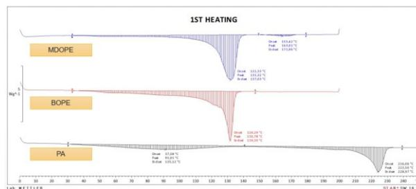
**Figure 5.** DSC analysis of outer layer PA, MDO-PE, and BOPE: 1<sup>st</sup> heating cycle
