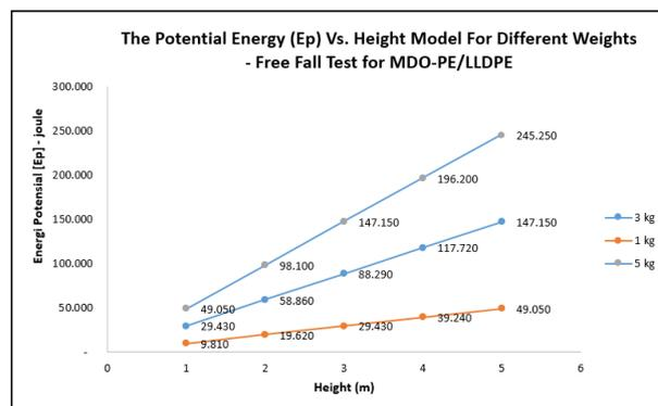
Figure 9. Potential energy (Ep) vs. height model for different weights – MDO-PE/LLDPE
