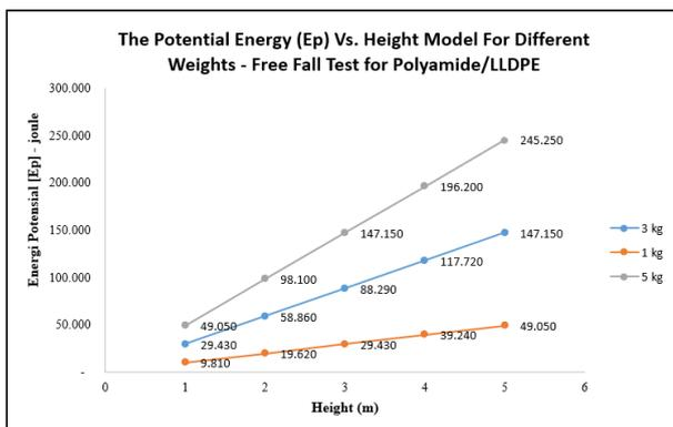
Figure 7. Potential energy (Ep) vs. height model for different weights – PA/LLDPE
