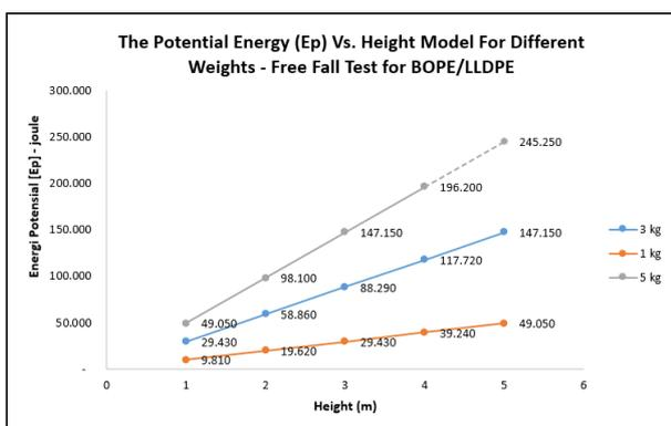
Figure 8. Potential energy (Ep) vs. height model for different weights – BOPE/LLDPE
