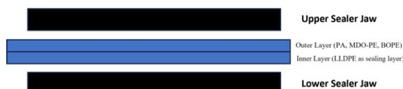
**Figure 3.** Illustration of heat resistances testing PA/LLDPE, MDO-PE/LLDPE, and BOPE/LLDPE
