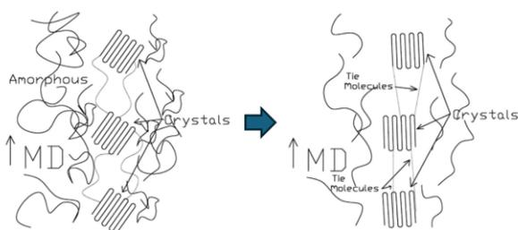
**Figure 4.** Mechanism of polymer molecular alignment [4]
