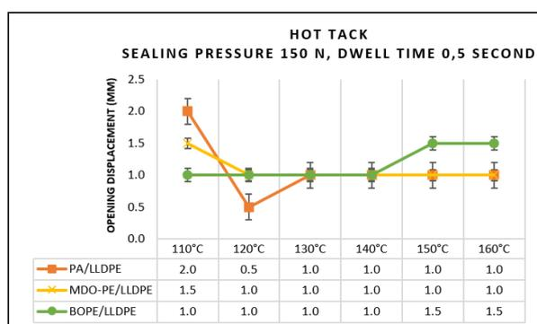
**Figure 2.** Hot tack performances (hermeticity seal) PA/LLDPE vs. MDO-PE/LLDPE vs. BOPE/LLDPE
