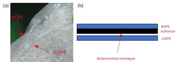
Figure 10. (a) Visual evidence of interlayer delamination in BOPE/LLDPE, (b) Schematic illustration of interlayer delamination in the structure of BOPE/LLDPE
