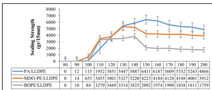
Figure 1. Sealing initiation temperature of PA/LLDPE, MDO-PE/LLDPE, and BOPE/LLDPE
