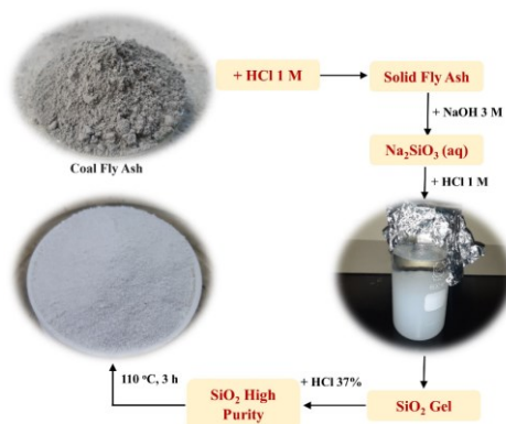
Figure 1. Schematic procedure for coal fly ash extraction
