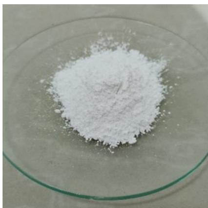
Figure 1. The appearance of the  $\text{Ca-Mg-NH}_4\text{-PO}_4$  composite from dolomite lime synthesis
