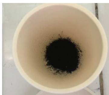
Figure 1. Activated carbon derived from styrofoam waste
