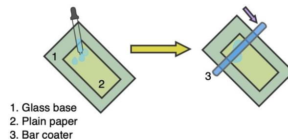
Figure 1. Bar coating process
