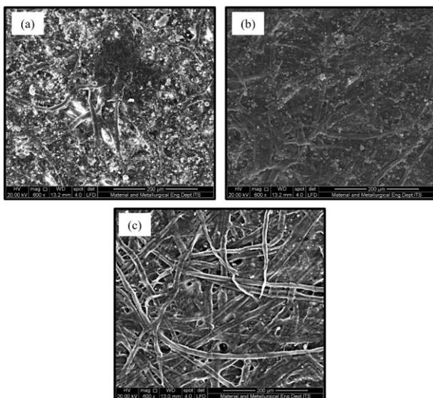
Figure 8. The surface SEM images of (a) 1% LMW chitosan-coated, (b) 2% LMWchitosan-coated paper, and (c) uncoated paper
