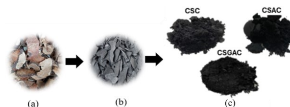
Figure 1. (a) Coconut shell, (b) Coconut shell charcoal/CSC, and (c) CSC, CSAC, CSGAC powder
