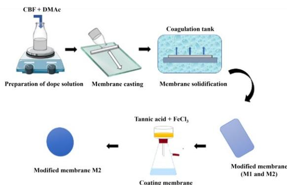
Figure 1. Membrane preparation
