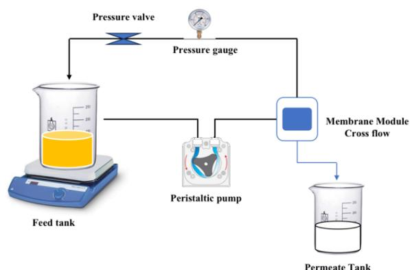
Figure 2. Filtration equipment setup
