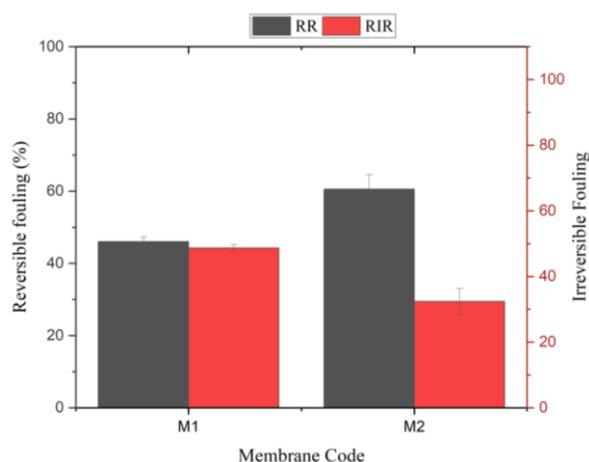
Figure 13.  $R_{ir}$  and  $R_r$  fouling values of the membrane
