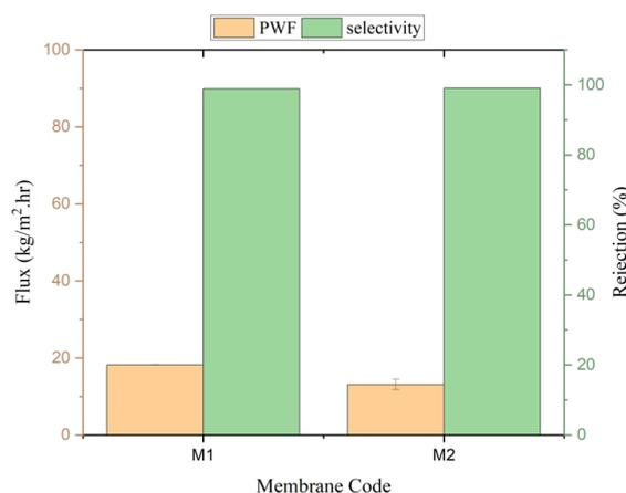
Figure 9. Pure water flux (PWF) and selectivity of the membrane
