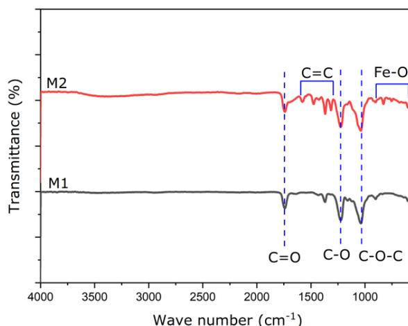
Figure 6. FTIR spectra of the membranes
