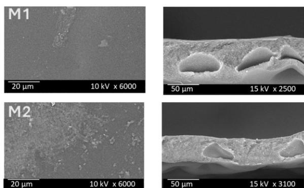
Figure 4. Surface and cross-sectional morphological structure of membranes
