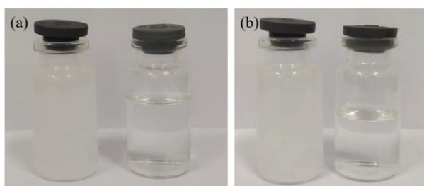
Figure 10. Oil emulsion filtration results (a) without additives and (b) with additives
