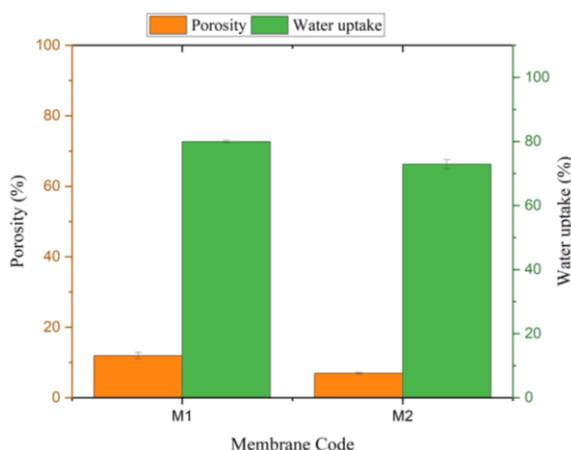
Figure 8. Water uptake and porosity of the membrane
