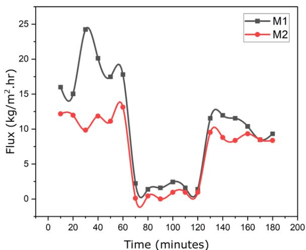
Figure 11. Flux decline and recovery profiles in the membranes
