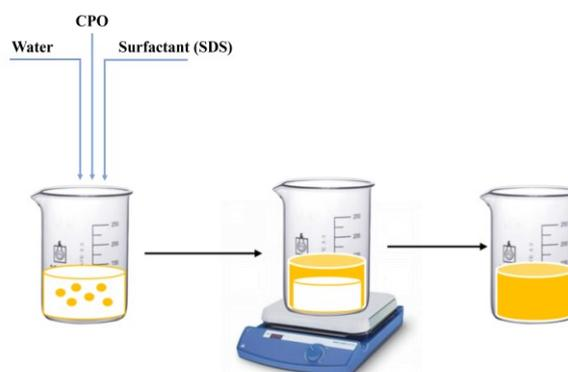
Figure 3. Preparation of artificial oil emulsion solution
