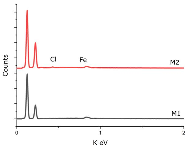
Figure 5. EDS spectrum of the membrane surface
