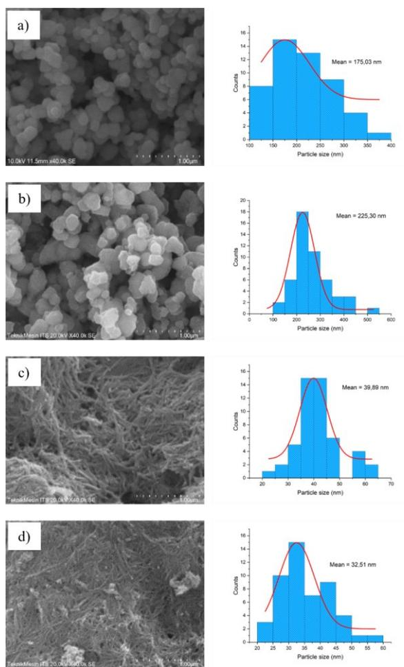
Figure 1. SEM images and particle size distribution of (a) anatase TiO<sub>2</sub> precursor, (b) rutile TiO<sub>2</sub> precursor, (c) TNPs(a), and (d) TNPs(r)
