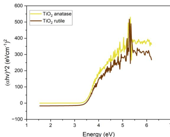
Figure 5. Tauc plot of TNTs versus photon energy
