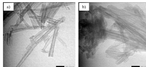
Figure 3. TEM images of (a) TNTs(a) and (b) TNTs(r)
