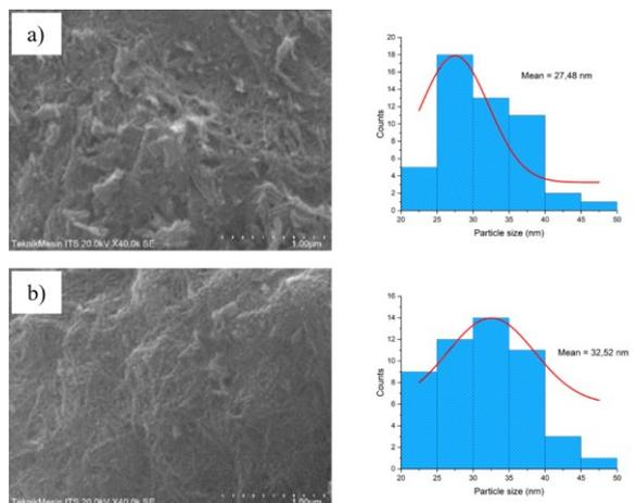
Figure 2. SEM images and particle size distributions of (a) TNTs(a) and (b) TNTs(r)
