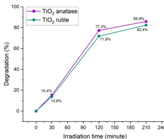
Figure 6. Graph of percent degradation of diazinon versus irradiation time
