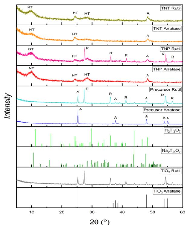
Figure 4. XRD diffractogram of TNTs (A = anatase, R = rutile, NT = sodium titanate, HT = hydrogen titanate)
