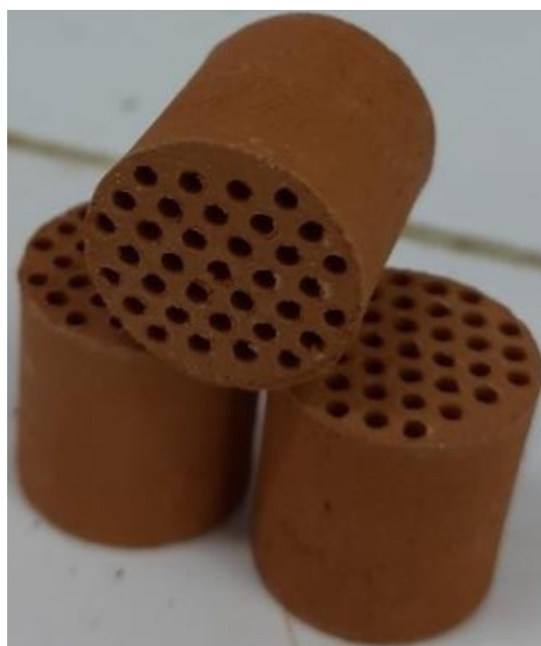
Figure 2. CBM product prepared using the mold method
