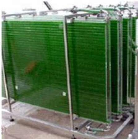
Gambar 3. Instalasi flat photobioreactor
