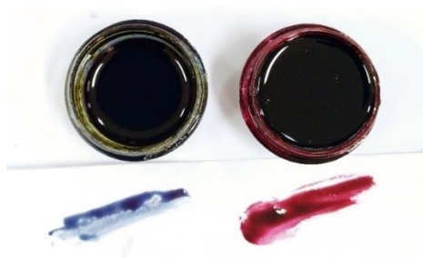
Figure 1. Visual appearance of butterfly flower extract using ethanol (blue color) and a combination of ethanol-citric acid (red color).
