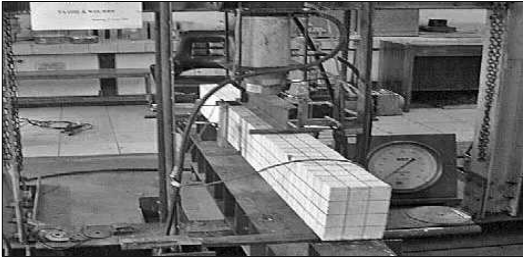
Figure 3. Beam specimen prior to loading
