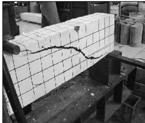
Figure 5 and 6. Normal and slag-concrete beam in shear failure
