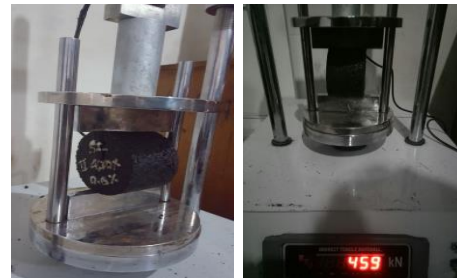
Gambar 7. Model pengujian ITS
