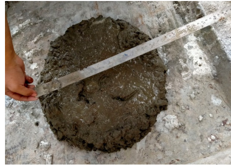
Gambar 3. Pengujian slump flow beton SCC
