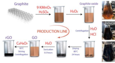
Figure 2. Production scheme using graphite powder as initial material. The provided image shows graphene oxide (GO), graphene oxide with citric acid (GO+CA), and reduced graphene oxide (rGO) (Tene et al., 2020)
