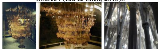
Figure 6. Gaudi's Sagrada Familia Structure Study Model Source: (De Luca, 2018)
