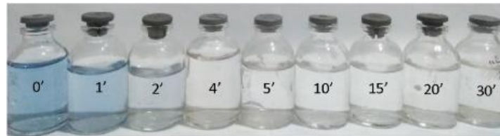
Figure 4. Removal of dye RB5 with a concentration of 5 mg/L with an ozone rate of 16.44 mg/minute
