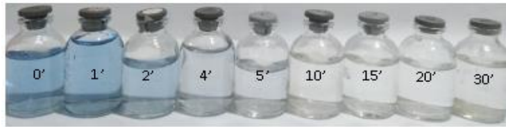
Figure 3. Removal of dye RB5 with a concentration of 5 mg/L with an ozone rate of 8.22 mg/minute
