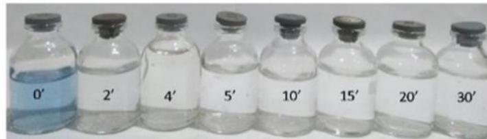
Figure 5. Removal of dye RB5 with a concentration of 5 mg/L with an ozone rate of 24.66 mg/minute
