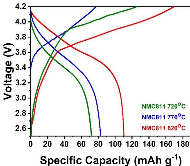
Figure 5. The charge-discharge of the NMC8<sub>11</sub> cathode material at 0.1C
