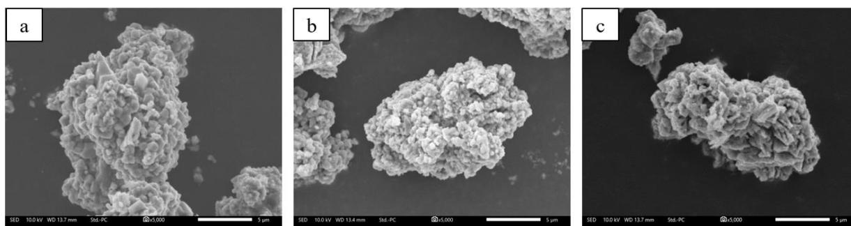
**Figure 4.** The SEM image of the NMC811 cathode material at various temperatures, (a)  $720^\circ\text{C}$ ; (b)  $770^\circ\text{C}$ ; (c)  $820^\circ\text{C}$
