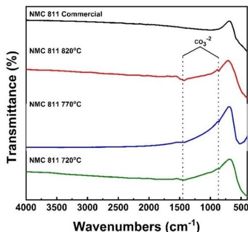
**Figure 3.** The FTIR peak of the NMC8<sub>11</sub> cathode material at various temperatures
