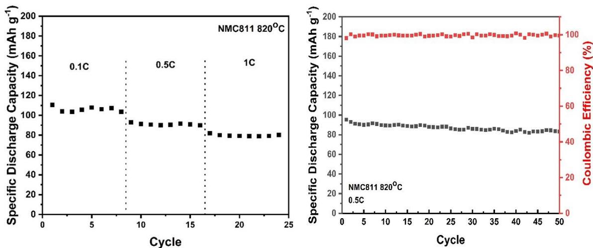
Figure 6. a) The rate-ability of the NMC8<sub>11</sub>; b) The cycle-ability of the NMC8<sub>11</sub>
