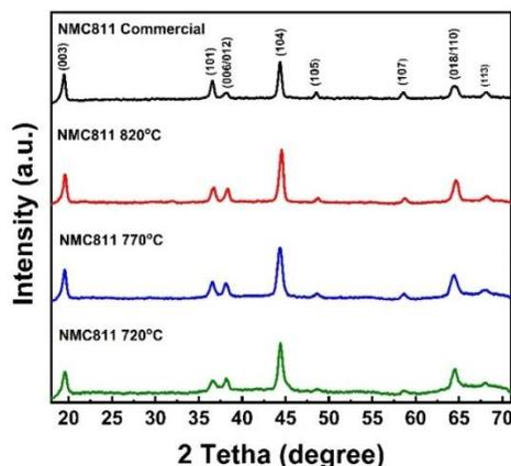
Figure 2. The x-ray diffraction pattern of the NMC811 cathode material at various temperatures
