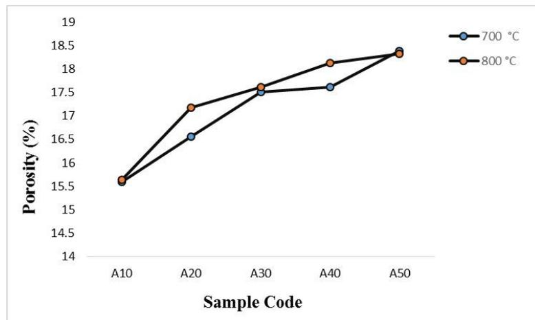
**Figure 1.** The relationship between composition variation and heating temperature on the porosity of red bricks
