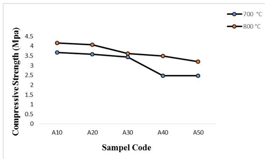
**Figure 4.** The relationship between variations in composition and heating temperature on the compressive strength of red bricks
