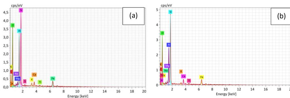
**Figure 8.** (a) Red brick EDS spectrum with sample code A10. (b) Red brick EDS spectrum with sample code A50
