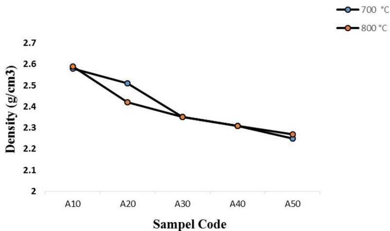
**Figure 2.**The relationship between composition variation and heating temperature on the density of red brick
