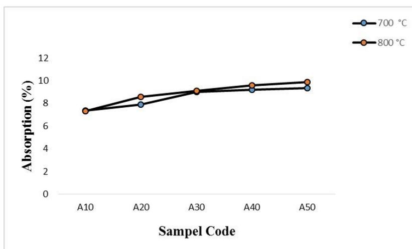
**Figure 3.** The relationship between composition variation and heating temperature on the absorption of red brick.
