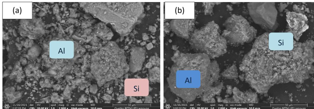
**Figure 6. (a)** The results of the morphology of the red brick SEM with the sample code A10. **(b)** Results of red brick morphology with sample code A50
