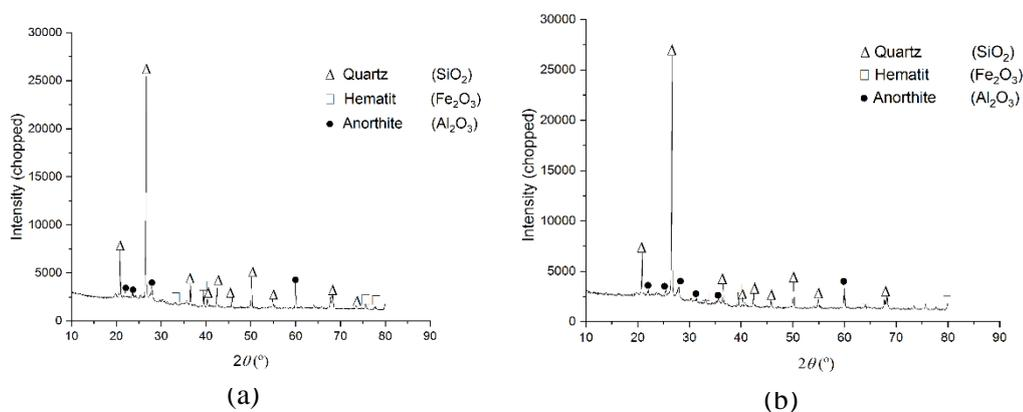
**Figure 5.** (a) Red brick XRD diffractogram with sample code A10; (b) Red brick XRD diffractogram with sample code A50
