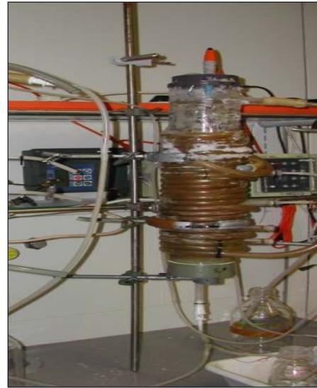
**Gambar 3.** (a) Skema Fixed-Bed Reactors (FBR), (b) Foto dari Fixed-Bed Reactors (FBR)
