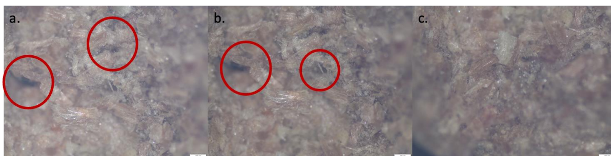
Figure 3. Digital Microscope observation for pellet with drying time a. 10 minutes, b. 15 minutes and c. 20 minutes (5x magnification)
