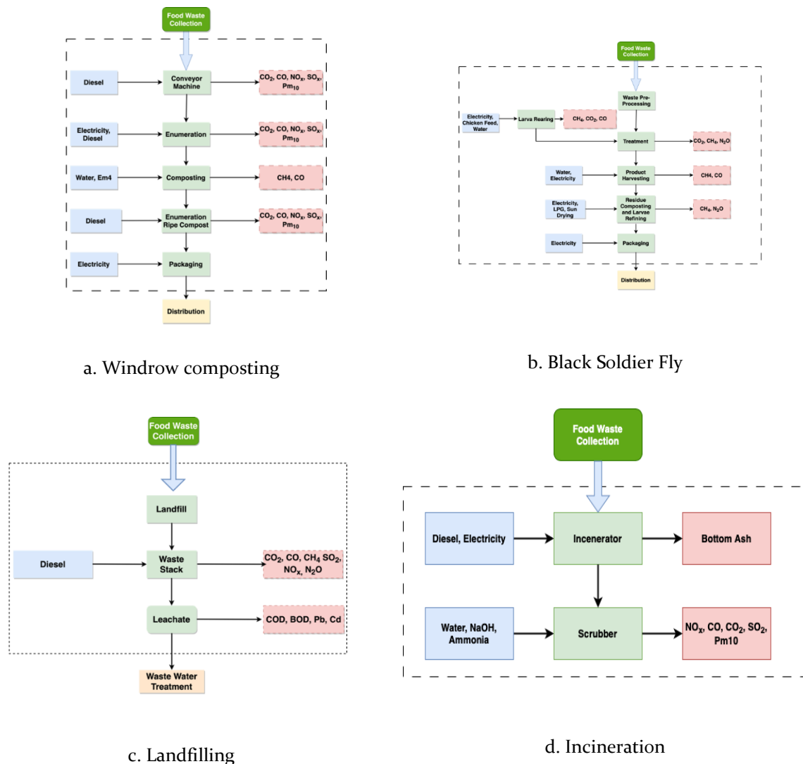
Figure 1. Flowchart showing the main processes involved in the four-system food waste management, a: windrow composting, b: Black soldier fly, c: Landfilling, and d: Incineration
