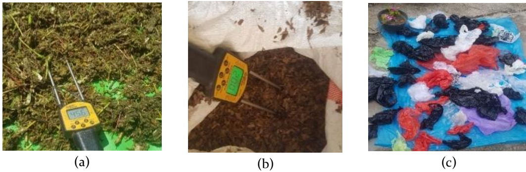
Figure 3. Drying and MC measurement (a) vegetables and fruit scraps (b) dry leaves (c) LDPE plastic waste
