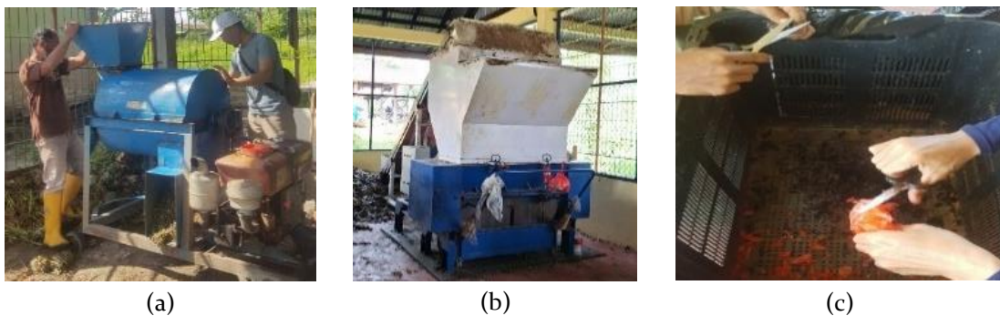
Figure 2. (a) Shredding vegetables and fruits (b) Shredding dry leaves (c) Shredding LDPE plastic waste
