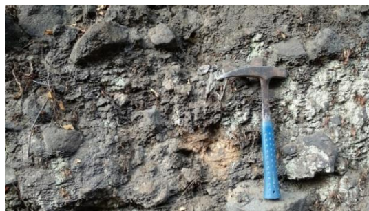
Figure 6. Lithology documentation of volcanic breccia (Coordinate 435790, 9222271)
