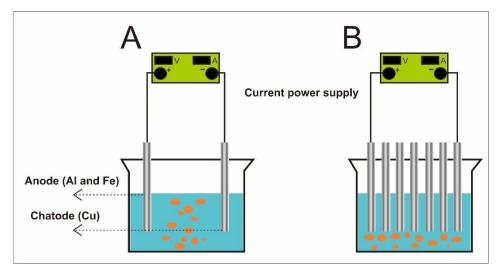
**Figure 5.** Electrocoagulation method for MPs removal (A) Monopolar electrode and (B) Biopolar electrode
