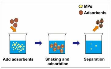
Figure 3. Schematic of MPs removal by adsorption process
