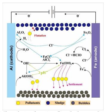
**Figure 6.** The mechanism of removing pollutans by electrocoagulation technique.
