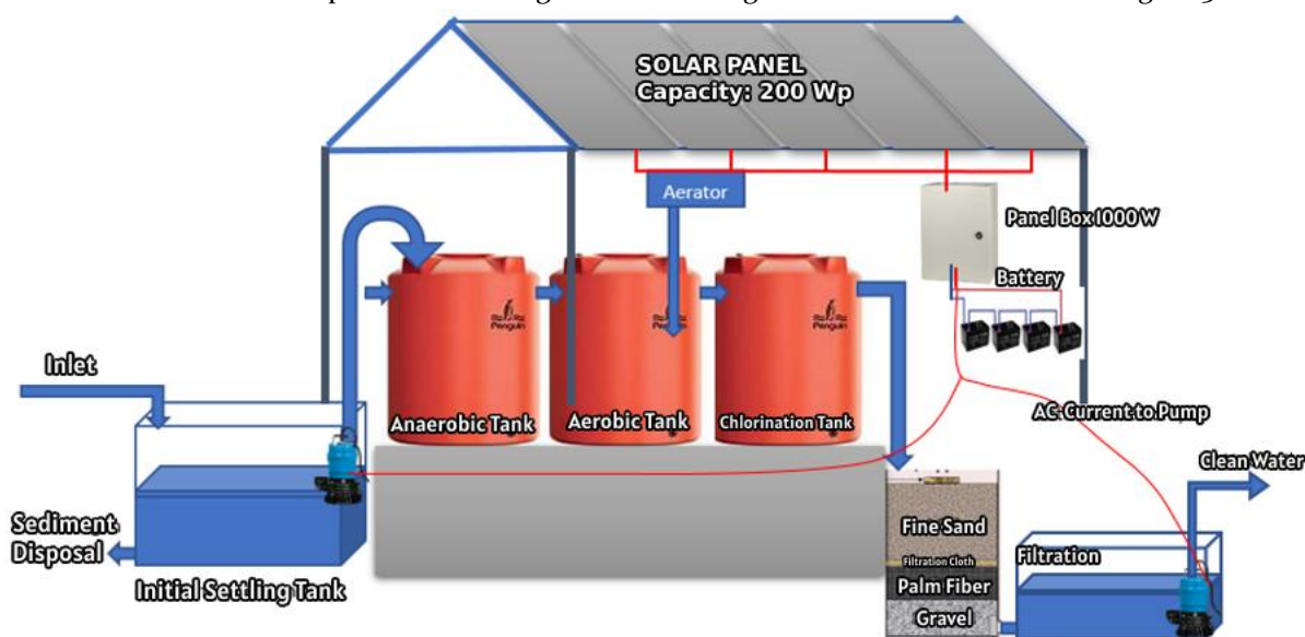
Figure 3. Wastewater treatment process diagram with a solar power-based anaerobic-aerobic biofilter process assisted by water filtration
