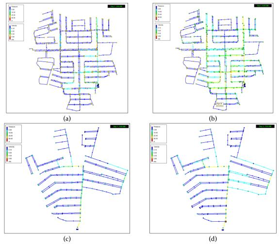
**Figure 2.** Epanet hydraulics simulation (a) Graha permata kota dma minimum hours (b) Graha permata kota dma peak hours (c) Elit kota mataram dma minimum hours (d) Elit kota mataram dma peak hour
