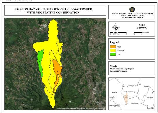
Figure 7. Erosion hazard index with conservation direction
