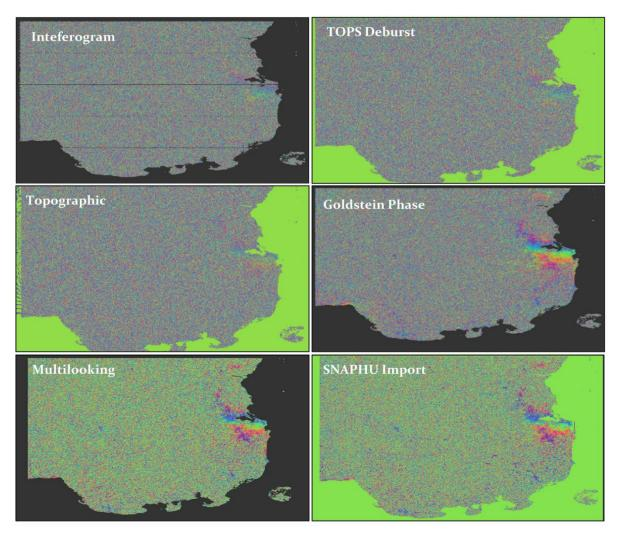
Figure 4. DInSAR processing steps using SNAP software
