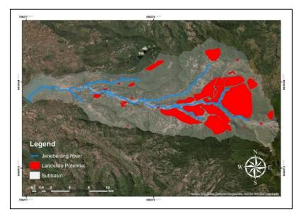
Figure 8. Landslide potential map of the Bili-Bili Reservoir catchment area
