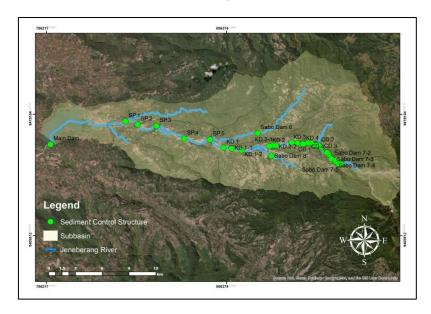
**Figure 9.** Map of existing sediment control structures in the Bili-Bili Reservoir catchment area Source: BBWS Pompengan Jeneberang (2020)
