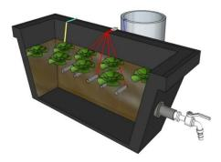
Figure 2. Reactor configuration with treatment of *Pistia stratiotes*
