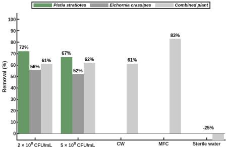
Figure 8. TSS removal efficiency in each treatment
