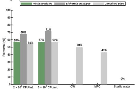
Figure 7. Ammonia removal efficiency in each treatment
