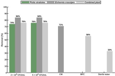
**Figure 5.** COD removal efficiency in each treatment
