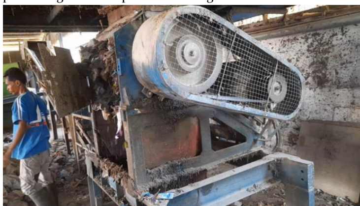
Figure 2. Crusher operated by local community to process dry mixed waste for RDF production
