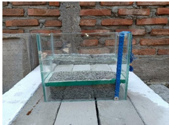
Figure 8. Falling head permeameter test equipment
