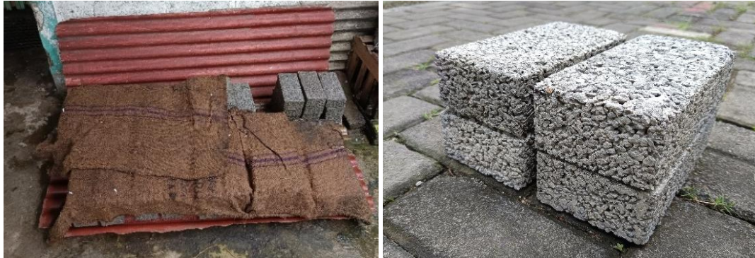
Figure 4. Curing process and pervious concrete paver block test objects.
