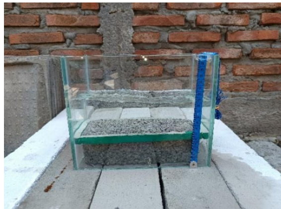
Figure 8. Falling head permeameter test equipment
