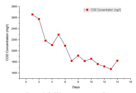
Figure 1. Daily COD concentration test reading
