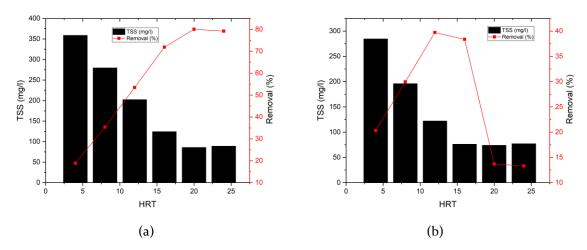
**Figure 5.** Removal % of total suspended solid (a)anaerobic and (b) aerobic from treated wastewater after biofilter process
