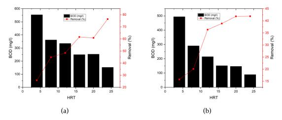
Figure 3. Removal % of BOD (a)anaerobic and (b) aerobic from treated wastewater after biofilter process
