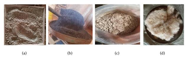
**Figure 1.** Materials used in the current study (a) expansive soil; (b) RHA; (c) lime; (d) sisal fiber
