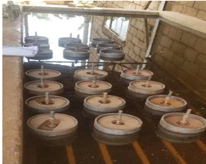
Figure 4. Soaking of compacted CBR specimens in a water tank
