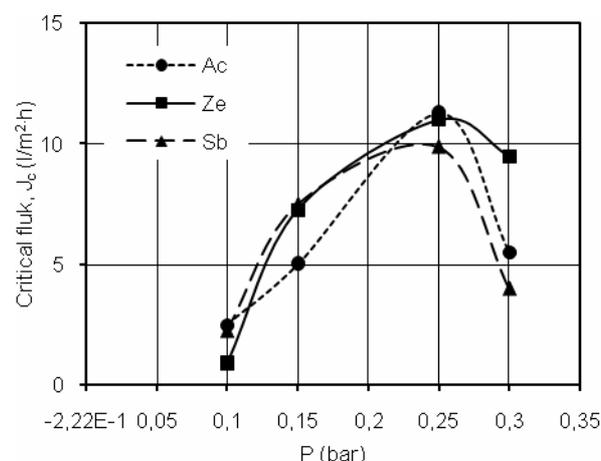
Figure 2. Effect of pressure on the critical flux for each MBR configuration
