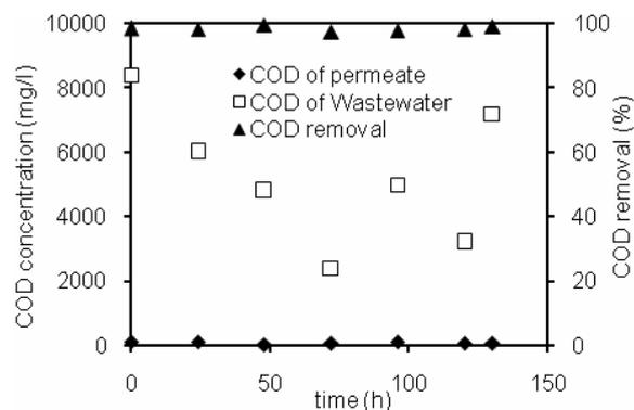
Figure 7. Rejection characteristics for Ac-eMBR in continuous mode
