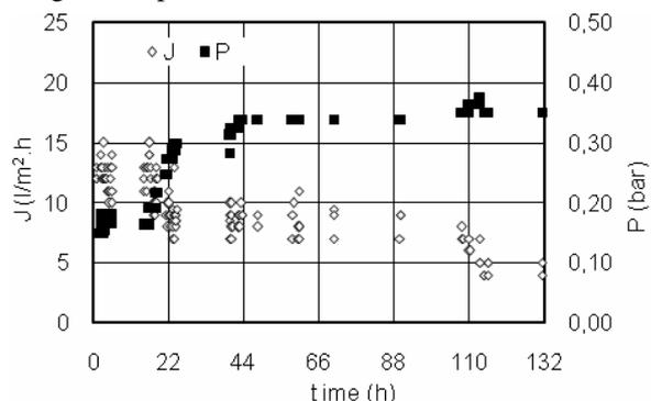
Figure 6. Relationship between flux and pressure for Ac-eMBR in continuous mode
