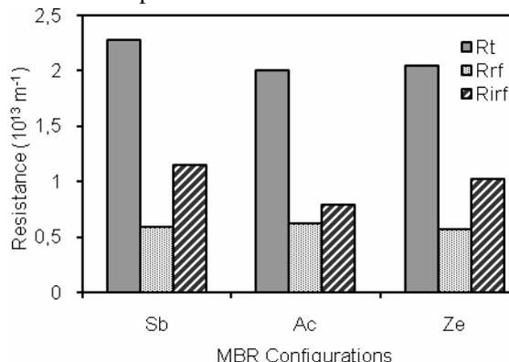
Figure 3. Series of resistance for each MBR configuration (Rt: total resistance; Rrf: reversible fouling; Rirf: irreversible fouling)
