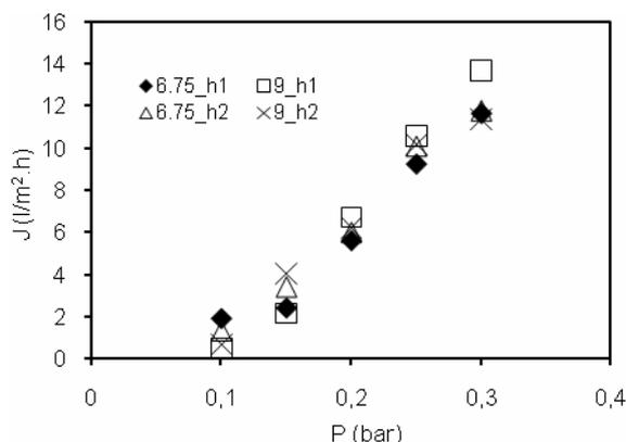
Figure 5. Profiles of stable flux of pure water at various bed thickness and aeration rate on TMP
