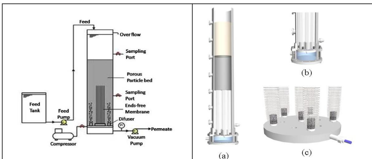
Figure 1. Schematic of newly configured submerged ends-free MBR (a: full-system; b: inner side of the MBR; c: air-flow pattern from diffuser located in the bottom of MBR)
