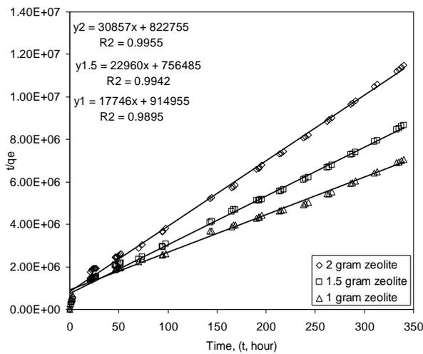
Figure 3. The second-order kinetics of Malachite Green adsorption on natural zeolite (T = 30°C)
