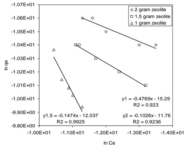
Figure 5. Freundlich isothermal plots for the removal of malachite green on natural zeolite (T = 30°C)
