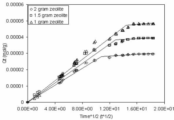
Figure 4. Intra particle diffusion modeling of malachite green adsorption on natural zeolite (T = 30°C)
