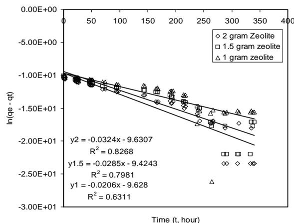
Figure 2. The pseudo-first-order kinetic of Malachite Green adsorption on natural zeolite ( $T = 30^\circ\text{C}$ )
