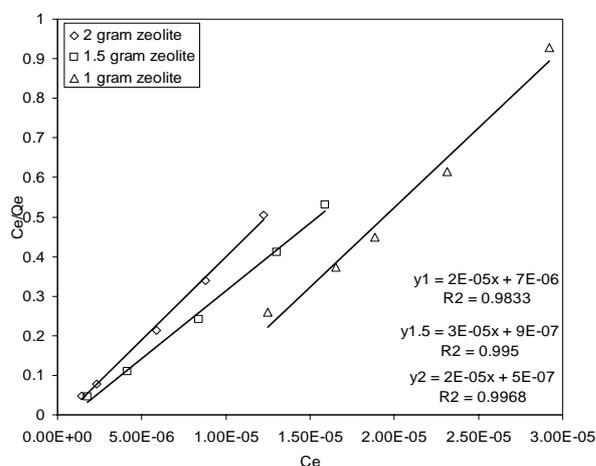
Figure 6. Langmuir isothermal plots for the removal of malachite green on natural zeolite ( $T = 30^\circ\text{C}$ ).
