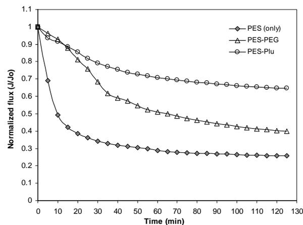
Fig. 7. Normalized flux during ultrafiltration of BSA solutions (0.1 g/L in phosphate buffer 0.05 M, pH 7) at a trans-membrane pressure of 300 kPa.
