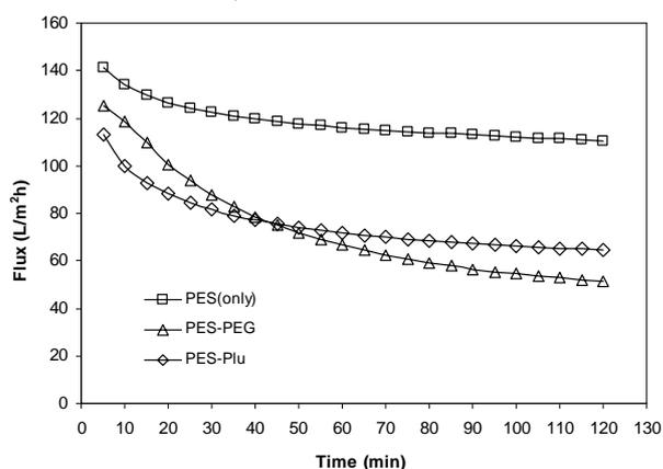
Fig. 2. Water flux profile over time during compaction at pressure of 450 kPa
