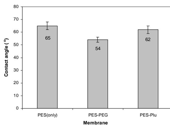
Fig. 4. Static contact angle (CA) measured by sessile drop method. The error bars represent standard deviation
