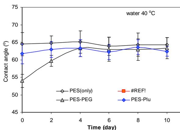
Fig. 8. Stability test in water (40°C) investigated by measuring the contact angle as a function of incubating time.
