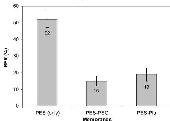
Fig. 6. Relative flux reduction after static adsorption using BSA (1 g/L in phosphate buffer 0.05 M, pH 7, 3 h exposure). The error bars represent standard deviation
