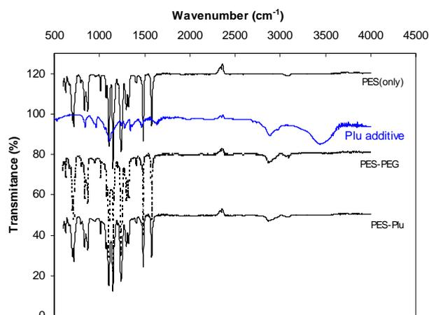
Fig. 5. FT-IR spectra of Pluronic additive and the membranes with different polymer composition
