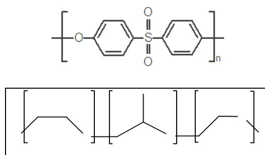
Fig. 1. Chemical structure of PES (top) and Pluronic (bottom) used
