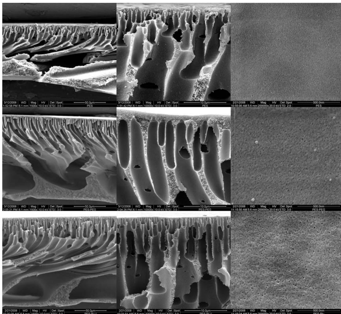
Fig. 3. SEM images of the cross section and membrane surface morphology: from the top to the bottom panel: PES (only), PES-PEG and PES-Plu, respectively.
