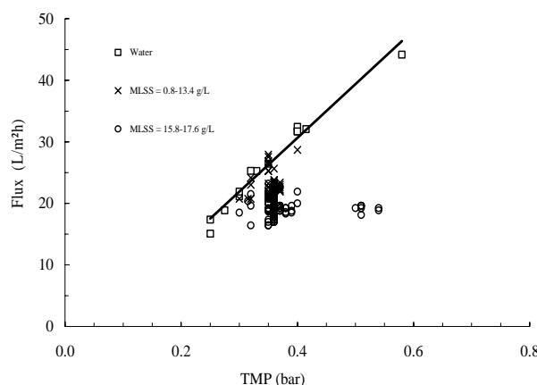
Figure 10. Flux versus transmembrane pressure of the ultratiltration operation
