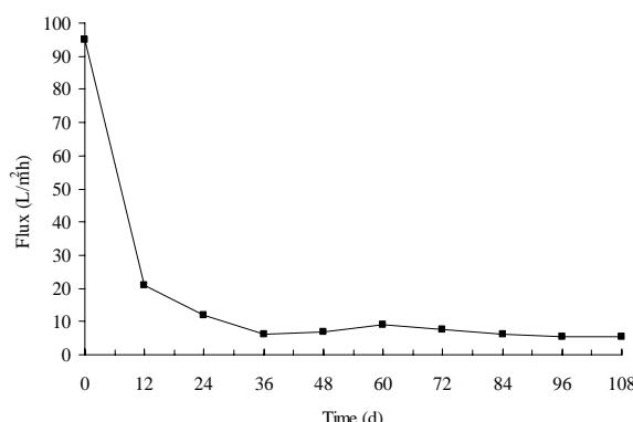
Figure 5. Permeate flux of the microfiltration membrane (leachate)
