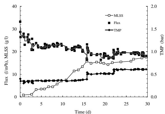
Figure 9. Profile of flux, pressure and MLSS over time of ultrafiltration
