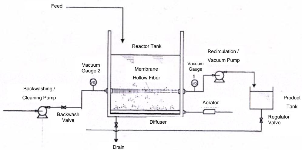
Figure 2. Schematic diagram of MF/UF-MBR for treatment of leachate
