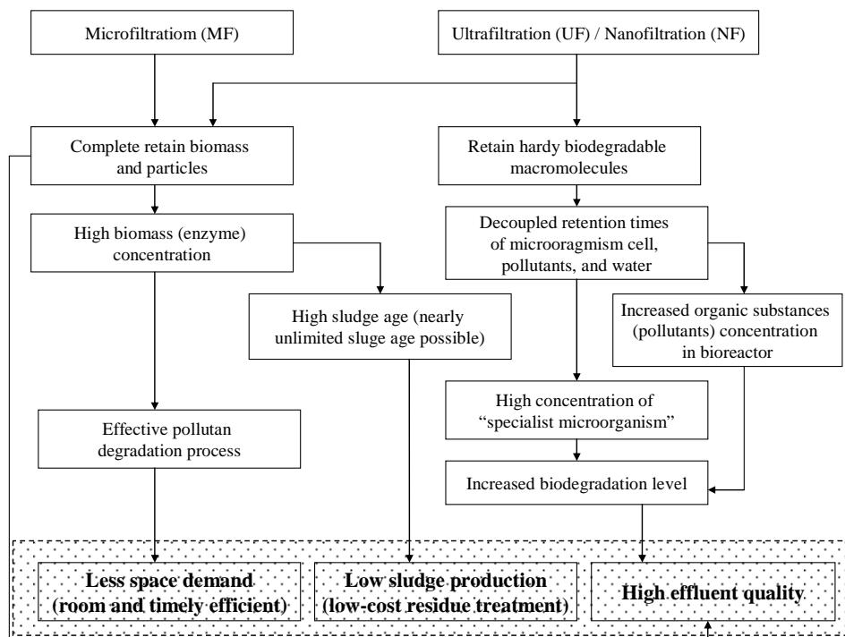
Figure 1. Effects of integration of a bioreactor with a membrane filtration in biological treatment system (Suprihatin, 1999)
