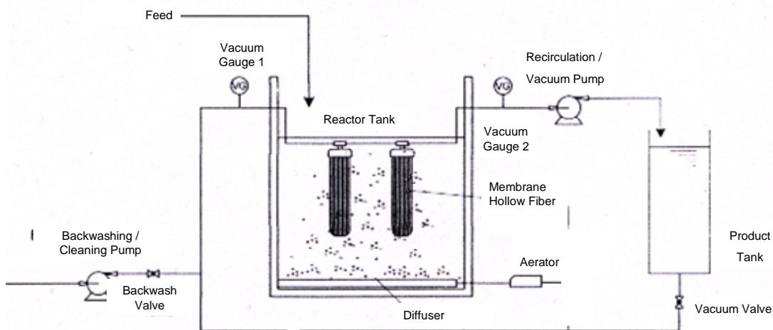
Figure 3. Schematic diagram of UF-MBR for treatment of pulp and paper mill effluent
