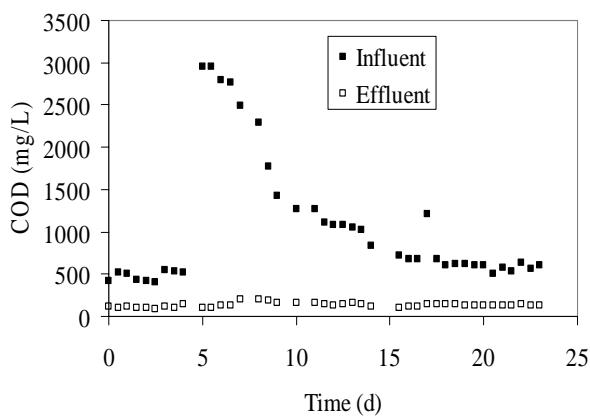
Figure 7. Performance of UF-MBR for treating pulp and paper mill effluent
