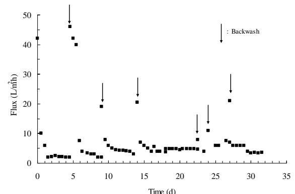
Figure 6. Effect of backwash on MF permeate flux
