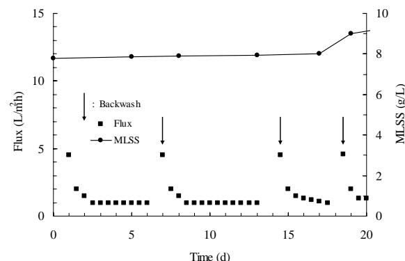
Figure 8. Permeate flux profile of UF membrane (pulp and paper mill effluent)
