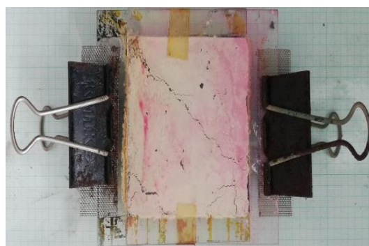
Figure 2. DSSC built in this study
