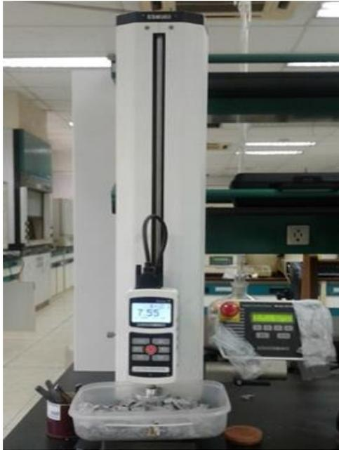
Figure 1. Compression tester for measuring granule crushing strength
