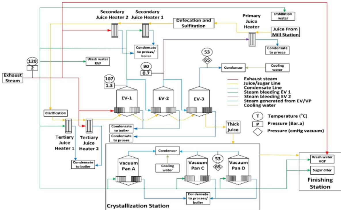
Figure 12. Sugar plant 4000 TCD thermal system diagram new integration works for MEE triple effect
