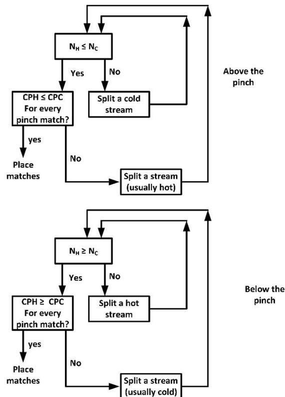
Fig 7. Algorithm for stream splitting at the pinch (B. Li *et al.*, 2019)
