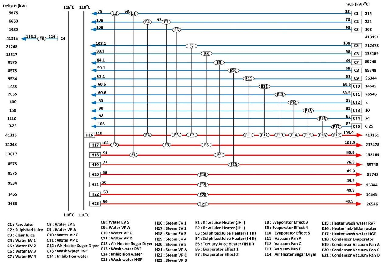
Figure 19. Heat Exchanger Network for new integration works MEE Quintuple Effect Evaporator
