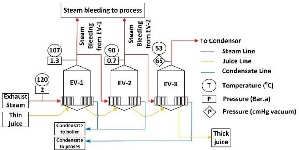
Figure 4. MEE Triple Effect Evaporator
