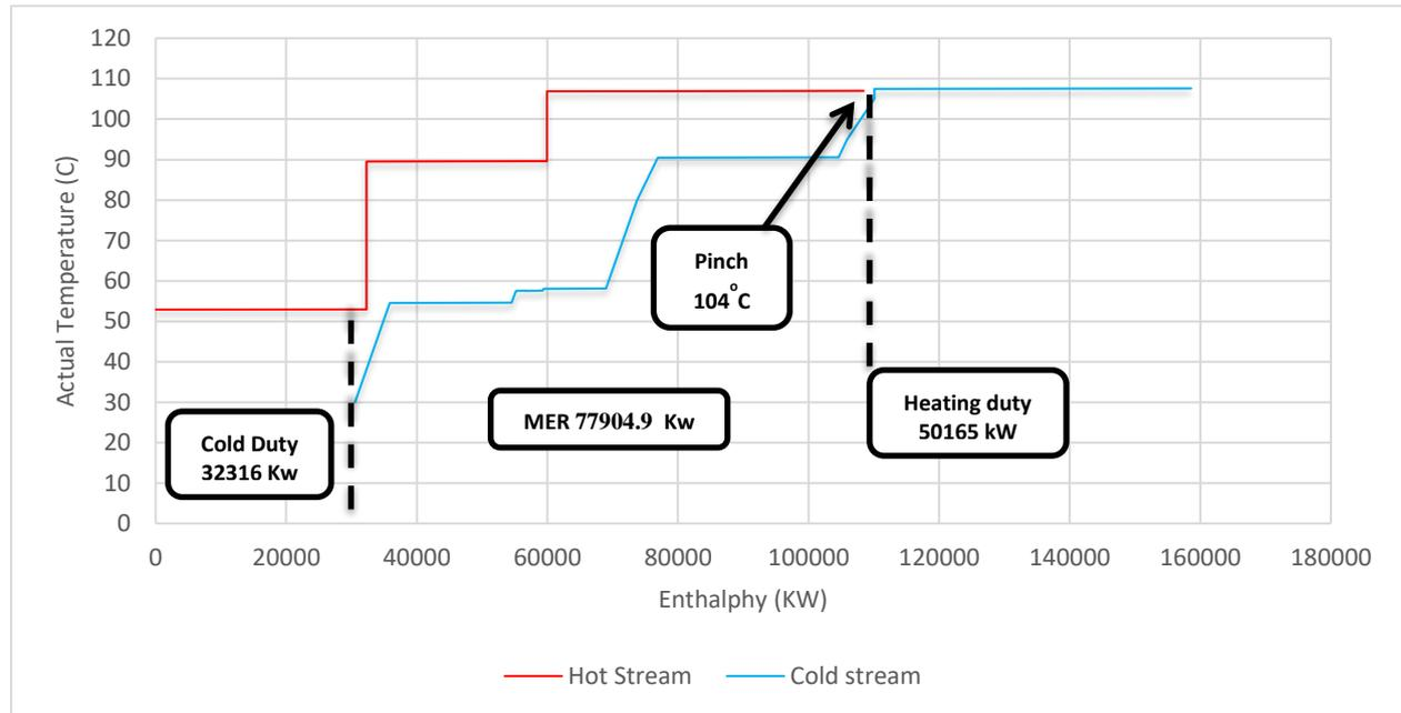
Figure 10. Composite Curve MEE Triple Effect Evaporator
