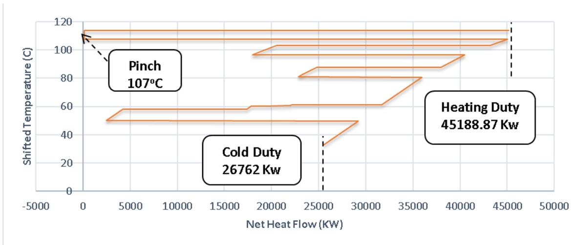
Figure 13. Grand Composite Curve MEE Quadruple Effect Evaporator
