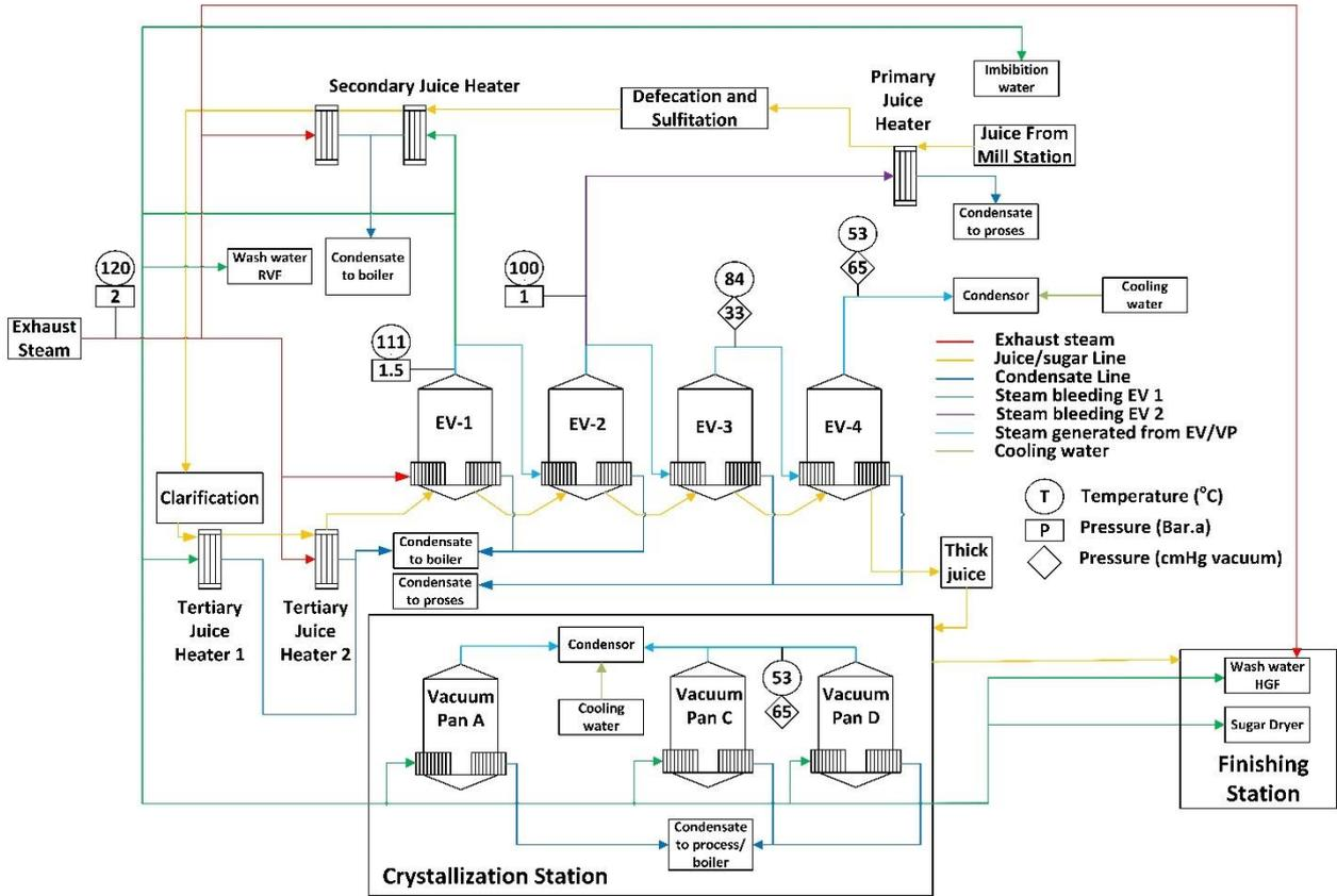
Figure 16. Sugar plant 4000 TCD thermal system diagram new integration works for MEE quadruple effect evaporator
