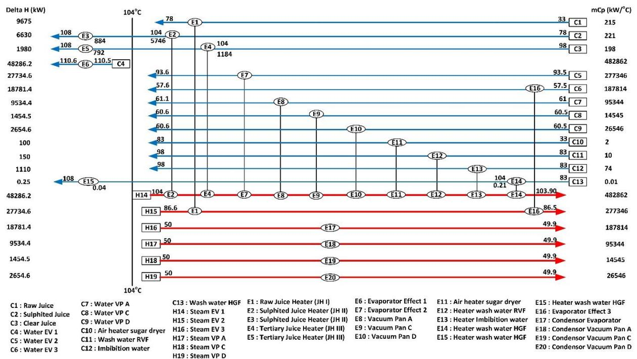
Figure 11. Heat Exchanger Network for new integration works MEE triple effect evaporator
