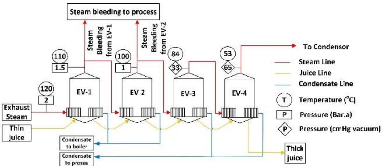
Figure 5. MEE Quadruple Effect Evaporator
