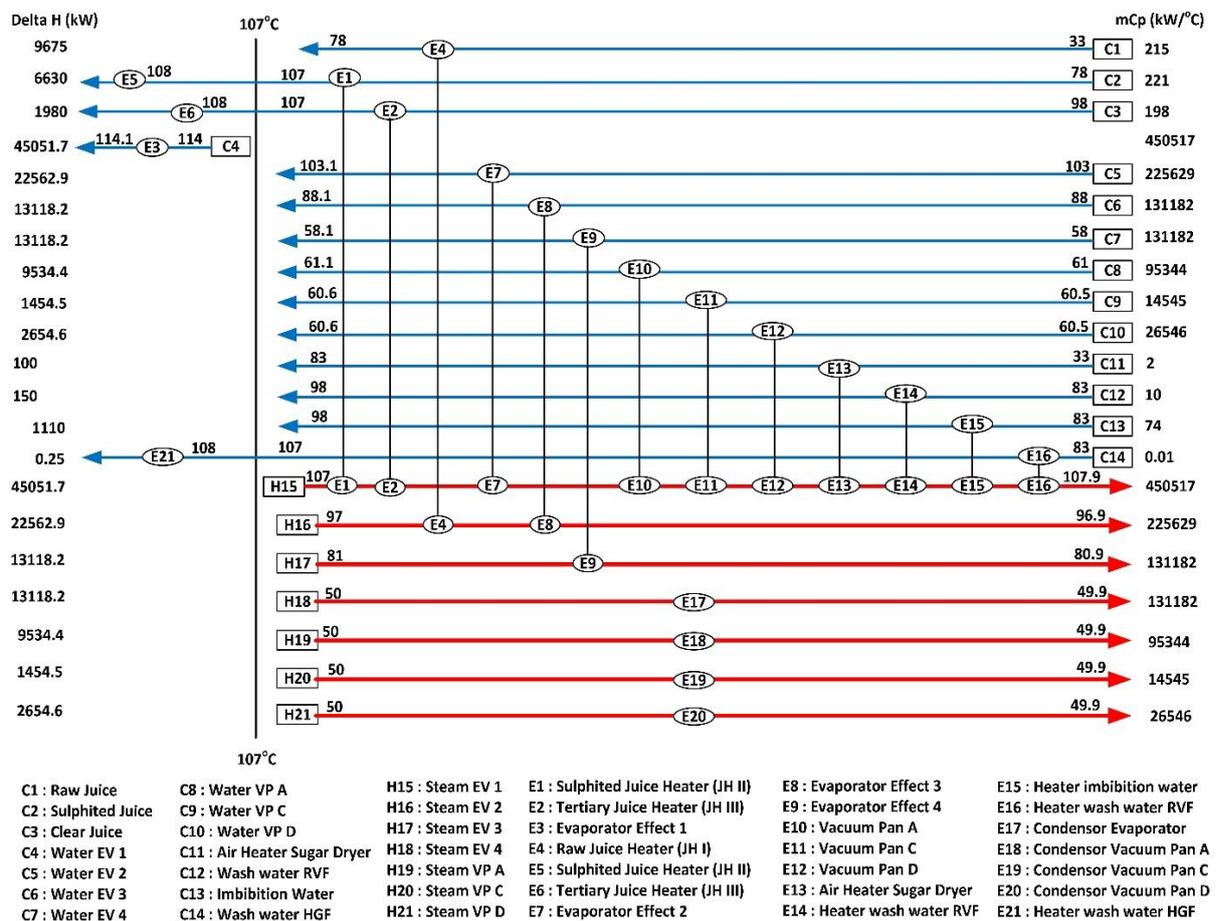
Figure 15. Heat Exchanger Network MEE Quadruple Effect Evaporator
