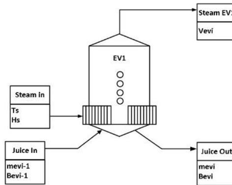
Figure 3. Evaporator effect i
