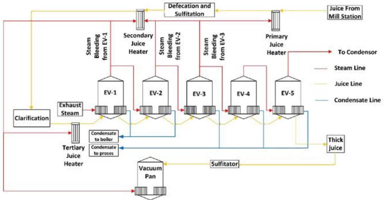
Figure 1. Process Flow Diagram Sulphitation Process Sugar Production
