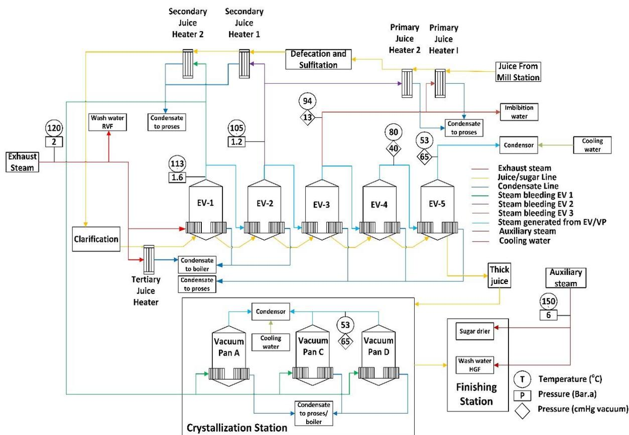
Figure 8. Sugar plant 4000 TCD thermal system diagram existing (MEE: Quintuple effect evaporator)
