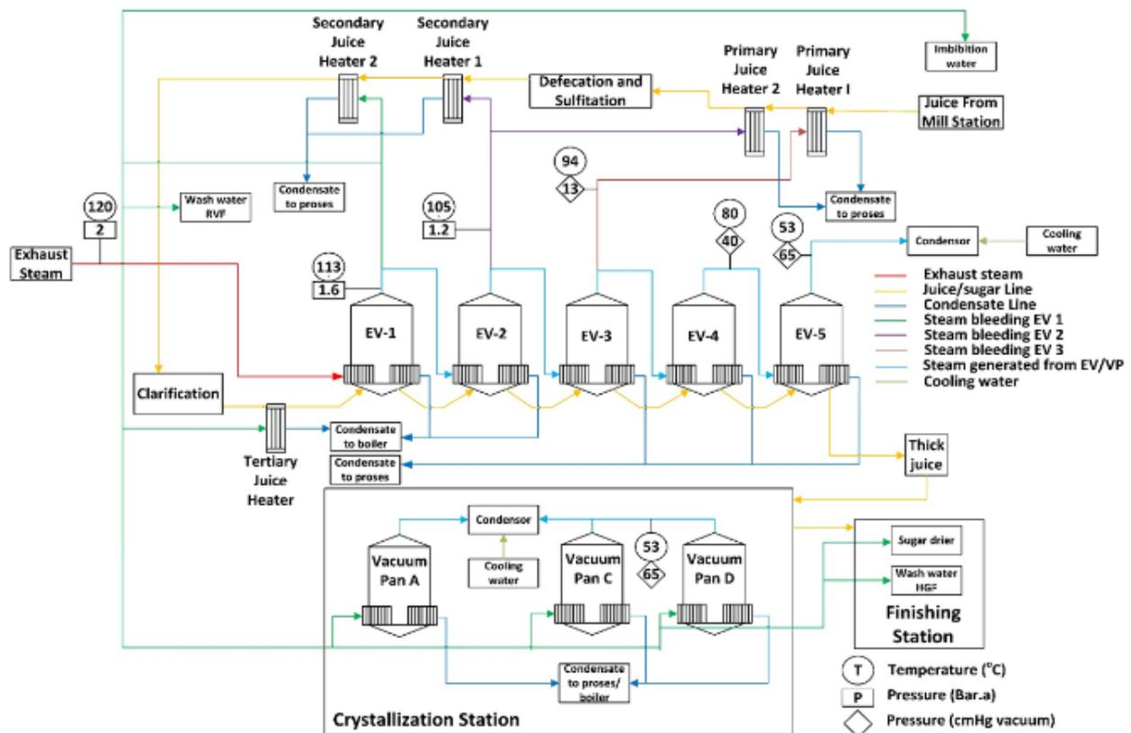
Figure 20. Sugar plant 4000 TCD thermal system diagram new integration works for MEE quintuple effect evaporator
