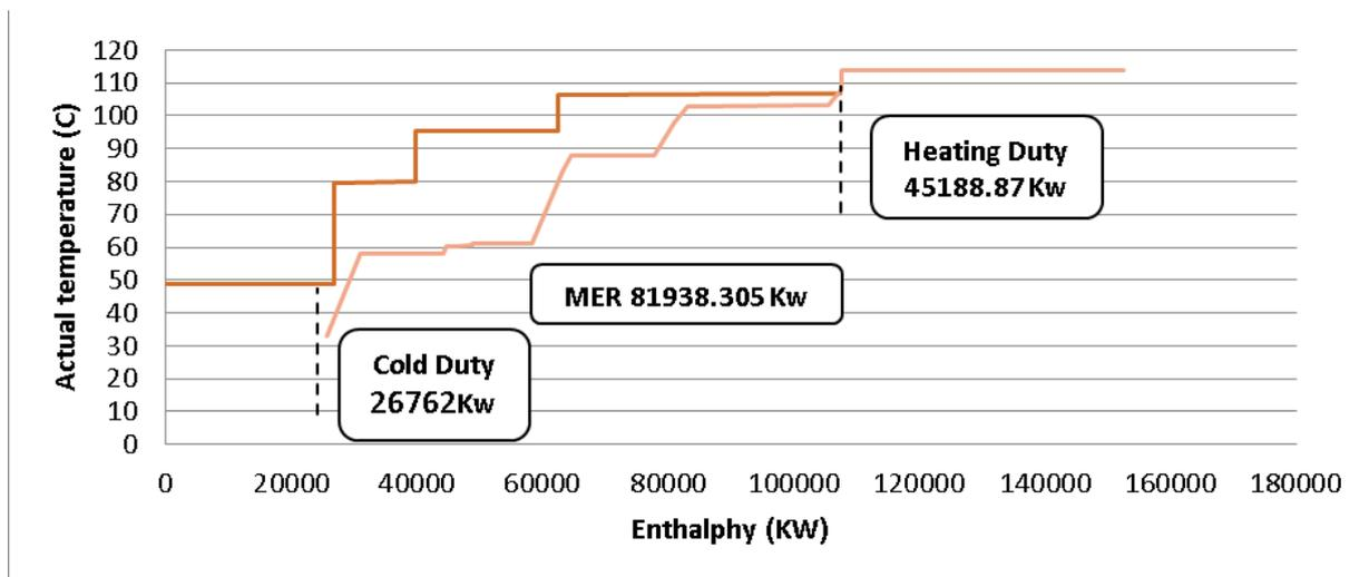
Figure 14. Composite Curve MEE Quadruple Effect Evaporator
