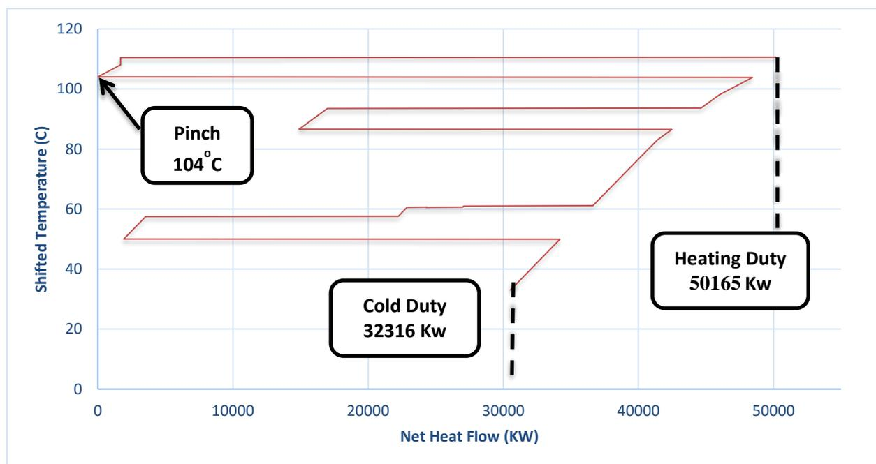
Figure 9. Grand Curve Composite MEE Triple Effect Evaporator
