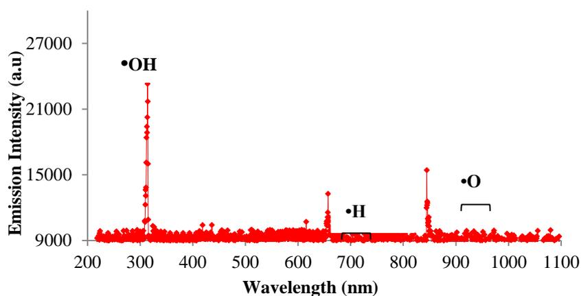
**Figure 4:** Radical Emission Intensity Without Air Injection
