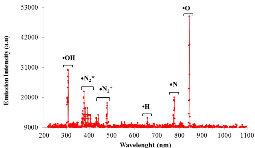
**Figure 5:** Radical Emission Intensity With Air Injection Flowrate 0.8 L.min<sup>-1</sup>
