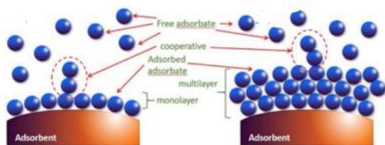
Figure 2. Layer of Adsorption in Interfacial Region, Monolayer, and Multilayer. Adapted from (Nandiyanto, 2020).
