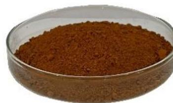
Figure 1. Non-magnetic bauxite Residue (200 mesh) after sieving
