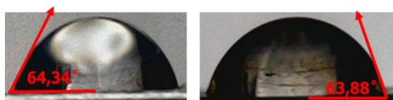
Figure 7. Contact angle measurement results (a) 70-SPSf 20 wt.%, HNT 1 wt.%, Acetone 6 wt.% (b) 98-SPSf 20 wt.%, HNT 1 wt.%, Acetone 6 wt.%
